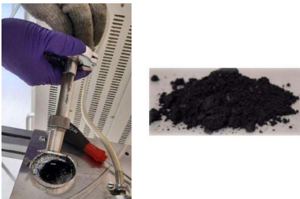
operation as soon as possible to help Taiwan achieve net-zero emissions by 2050. Figure 2.6.4 Results of Carbon Production from Methane Pyrolysis by Academia Sinica 158
